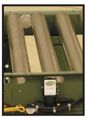
The combination of EZLogic® and EZDrive™ technology makes the 36-CREZD ideal for pallet storage and retrieval systems. When pallets are accumulated or not flowing on the conveyor the zones go into sleep mode. While in sleep mode, the zone stops running in order to save energy and save wear on mechanical components.
