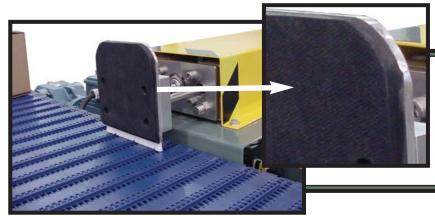
The ViperSort's pusher face is coated with rubber to provide gentle handling of products. Even products packaged in glass containers have been successfully sorted with the ViperSort.
