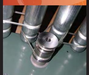
By replacing the drive spool with the optional limited slip spool assembly, E24<sup>TM</sup> conveyors can be used in minimum pressure applications. No other 24 VDC conveyor drive technology offers this unique capability.
