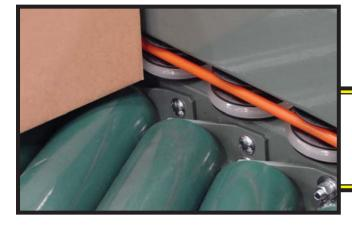
Powered Guide Rail in tooth area for accurately tracking cartons through merge
